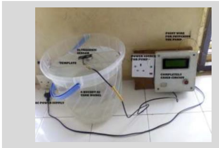
Figure 3: System ready for calibration.
