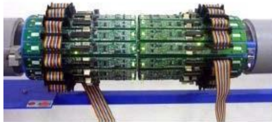
Figure11. A twin-plane segmented ECT sensor with 16 portable electrodes [24]
