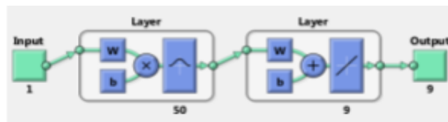
Figure 7. RBFNN structure for 10 bus system without DG
