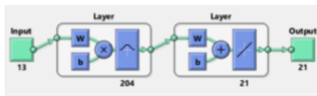
Figure 17. Structure of RBFNN for 34 bus system with DG
