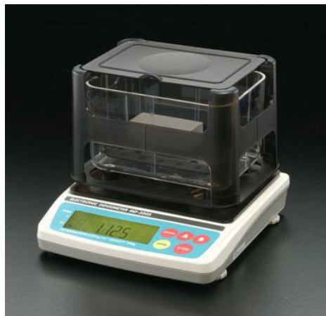
Figure 1. Figure show example of densimeter.
