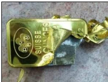
Figure 1. Fake gold bar that contains tungsten [12]
