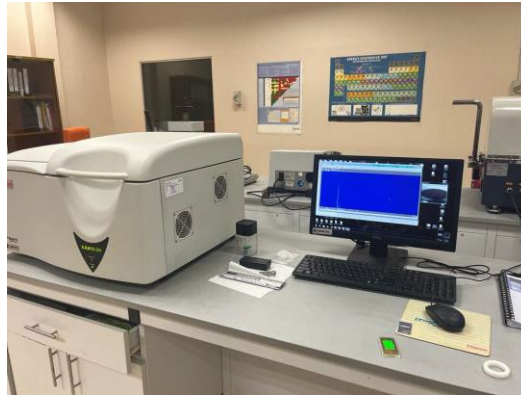
Figure 2.1 Setup for EDXRF and PC for experiment.
