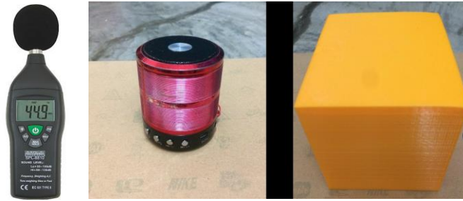
Figure 5. Sound Reductions Experimental Setup consists of Sound Level Meter, Wireless Speaker, and Acoustic Enclose Sample
