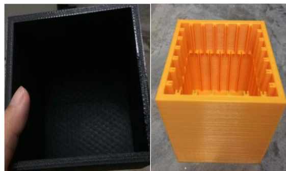
Figure 4. 3D Printed of (a) Acoustic Enclosure and (b) Acoustic Enclosure with Metamaterial
