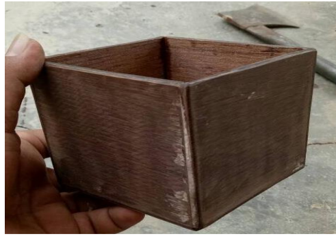
Figure 2. Wood Acoustic Enclosure with Dimension of 100 mm 3
