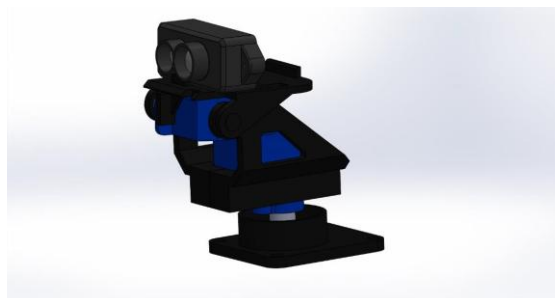
Figure 2. SOLIDWORK drawing of the servo-controlled gimbal with TF-mini LiDAR sensor
