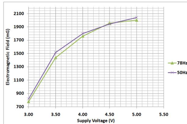
**Figure 4.1** Relationship between the voltage supplied to the coil circuit and the magnetic field produced
