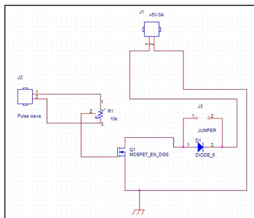
**Figure 3.8** Current Drive circuit
