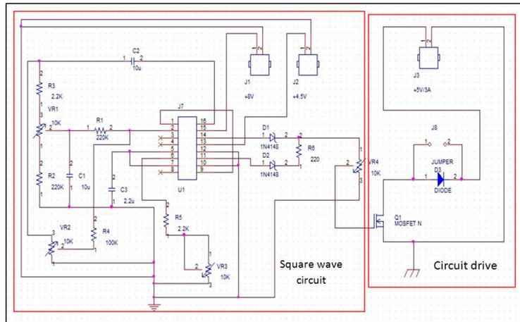
**Figure 3.6** Circuit Drive with IC UC3825 and Power MOSFET
