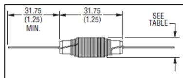
**Figure 3.3** Excitation coil dimensions
