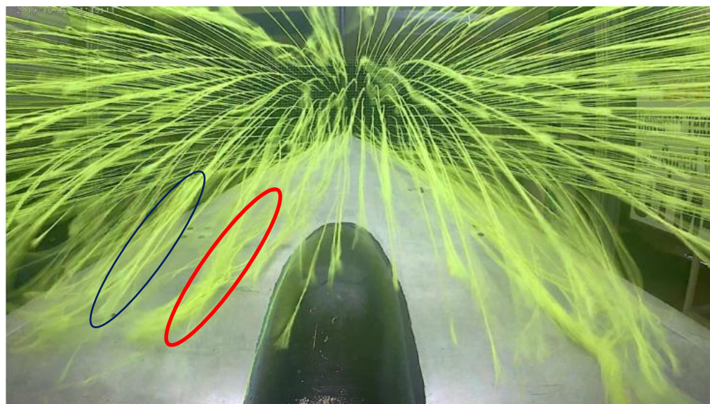
Figure 6. Flow visualization at angle 12.5°(medium leading edge, speed 18m/s)
