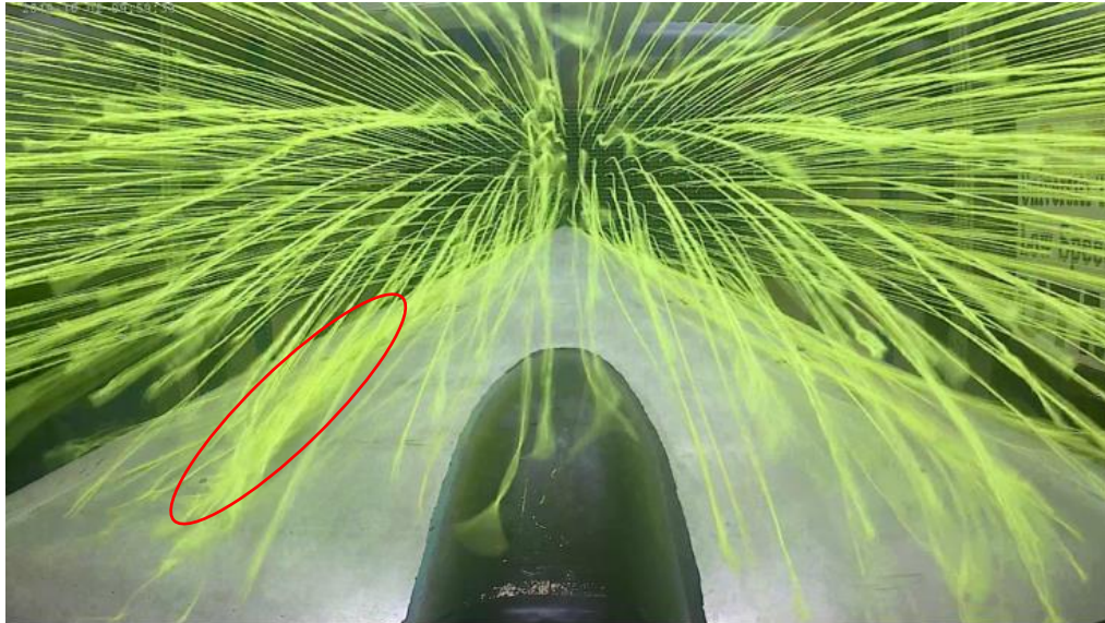
Figure 5. Flow visualization at angle 5°(medium leading edge, speed 18m/s)
