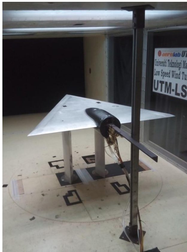
Figure 3. Installation of UTM VFE-2 model at \alpha=0^\circ
