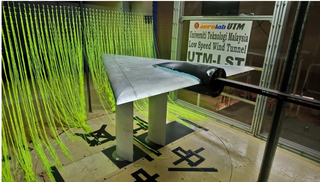
Figure 4. Tuft set up in front of the model
