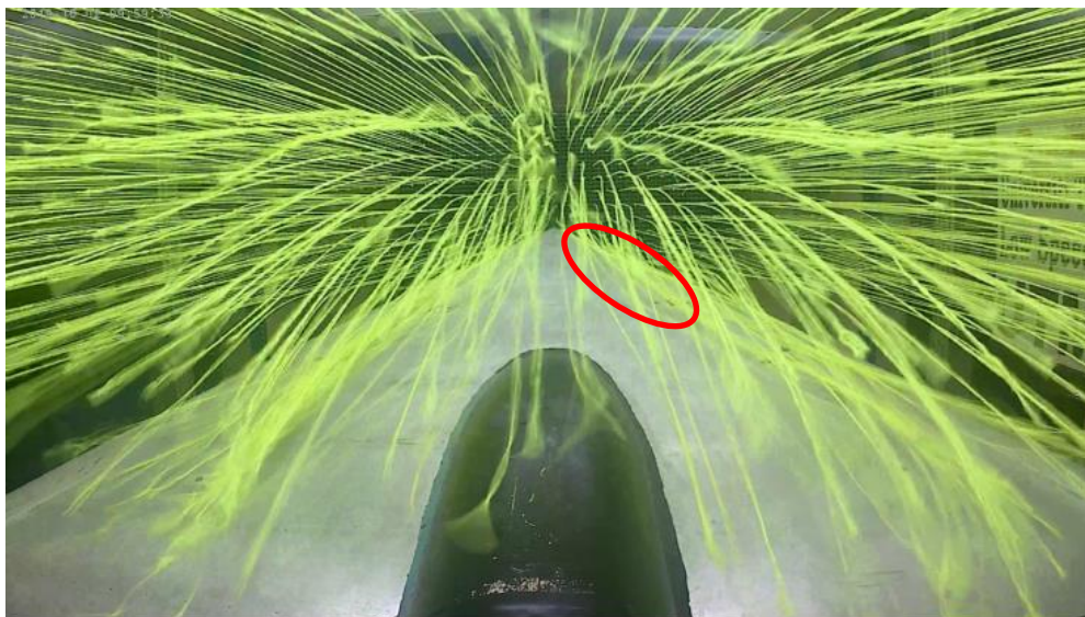
Figure 11 Flow visualization for medium-edged wing (speed at 18m/s, angle at 10°)
