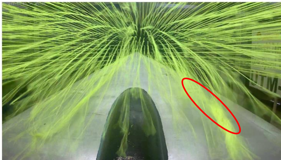
Figure 9. Flow visualization at Reynolds number of 2 \times 10^6 (medium leading edge, angle at 12.5^\circ )
