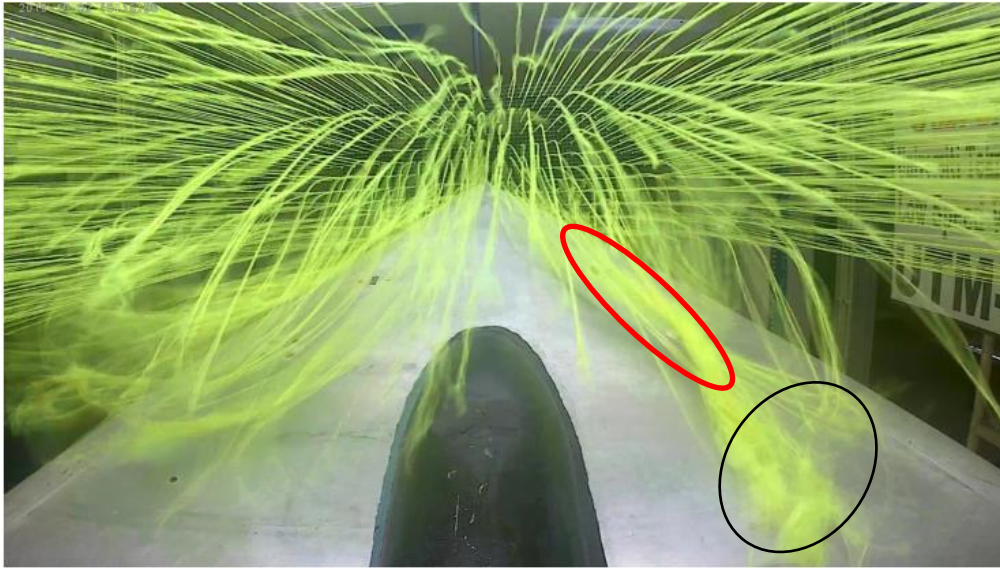
Figure 7. Flow visualization at angle 15^\circ (medium leading edge, speed 18m/s)
