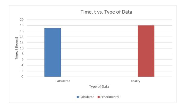
The graph above shows the difference between calculated time taken for battery to fully charge and the time taken on field test.
