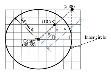
Figure 3. Example of illustration to eliminate pipe thickness
